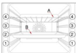
Inside the oven are side racks 1-4 for inserting the accessories A+B.
