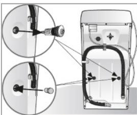
Remove the transport locking screws with a wrench. Insert the supplied transport locking covers.
