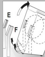
Remove the transport protection strips **E** and **F** (fixing the drum). For this tilt the appliance carefully forwards.
