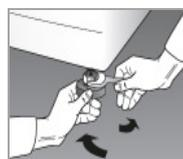
Use the wrench to loosen the lock nuts. Rotate the feet to change the height.
