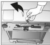
To do this, move the transport lever below the unit base to the left. Return the lever to its original position after determining the final location for the device.
