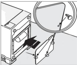
Align the plate in its intended position underneath the device and fix it with the enclosed clips.
