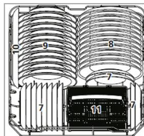
Because of the particularly intense cleaning action of the lower spray arm the lower basket is suitable for heavily soiled dishes. Load e.g. pots and plates.
