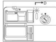
As long as the corresponding message does not light up in the display, you can estimate the amount of remaining rinse aid to the optical level indicator (D) next to the dispenser.
